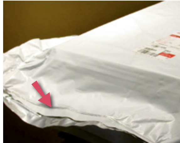
FIG 7 • Heat sealed line in foil packaging
