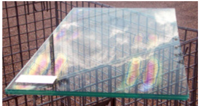
FIG 23 • Laminate showing optical distortion
