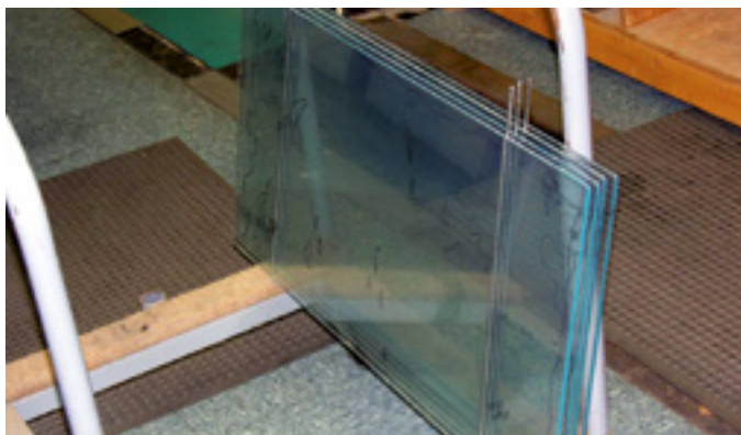
FIG 22 • Improperly racked laminates
