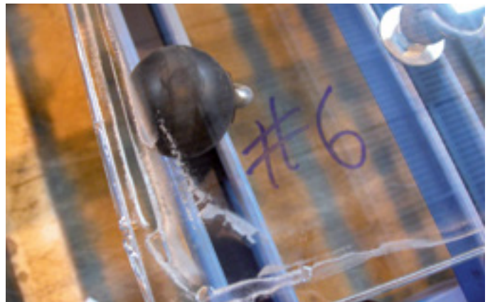
FIG 18 • Trapped air in trailing edge
