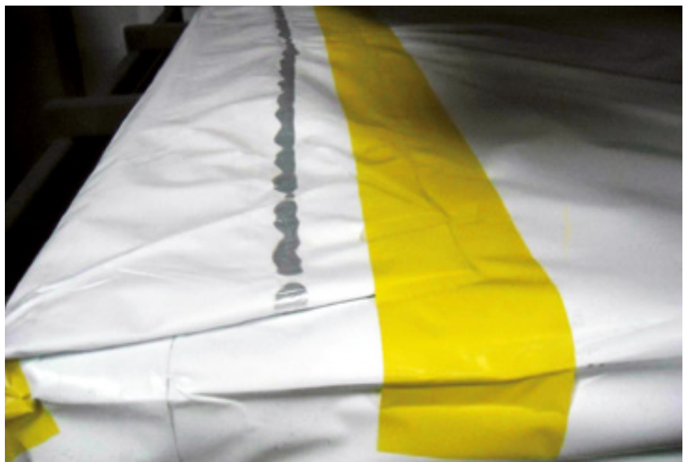
FIG 8 • SentryGlas® Xtra™ interlayer package – properly resealed with tape
