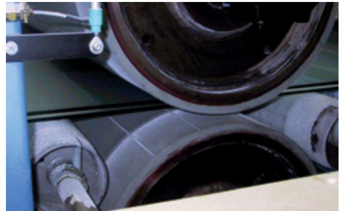
FIG 14 → Nip roll process
