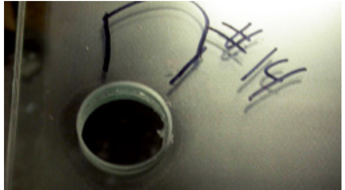
FIG 32 • Prepress too cold
