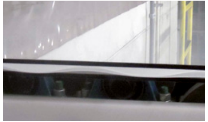
FIG 13 → Prepress interlayer waviness multiple sheets
