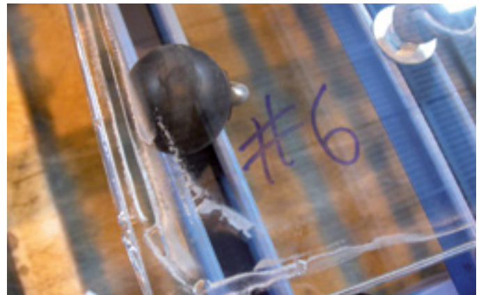
FIG 18 • Trapped air in trailing edge
