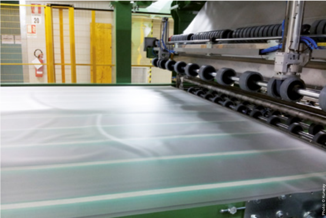
• PVB lay-flat behavior with Jumbo size glass laminates
