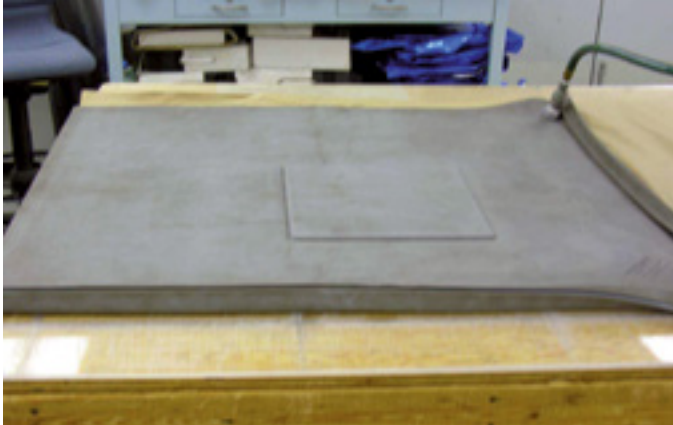
FIG 20 • Silicone rubber envelope bag (reusable)
