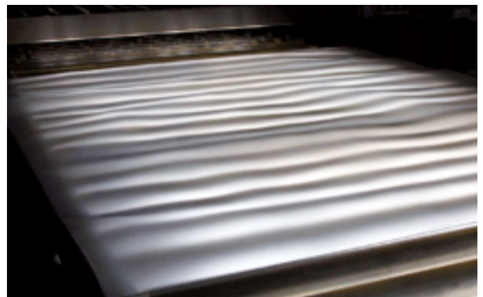
FIG 12 → Prepress interlayer waviness
