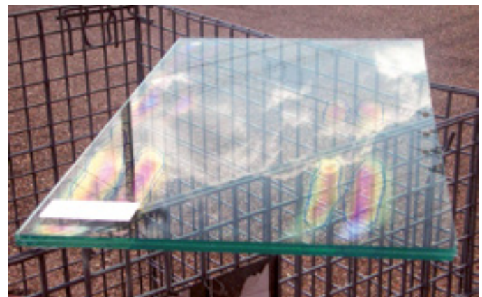
FIG 23 • Laminate showing optical distortion
