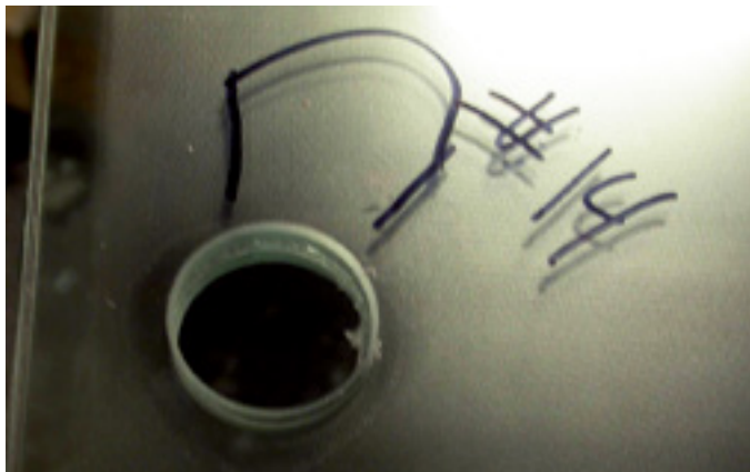
FIG 32 Prepress too cold
