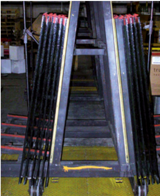
FIG 24 Properly racked laminates
