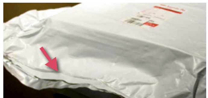
FIG 5 • Heat sealed line in foil packaging
