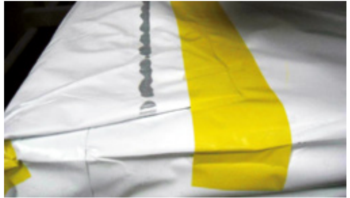
FIG 6 SentryGlas® interlayer package – properly resealed with tape
