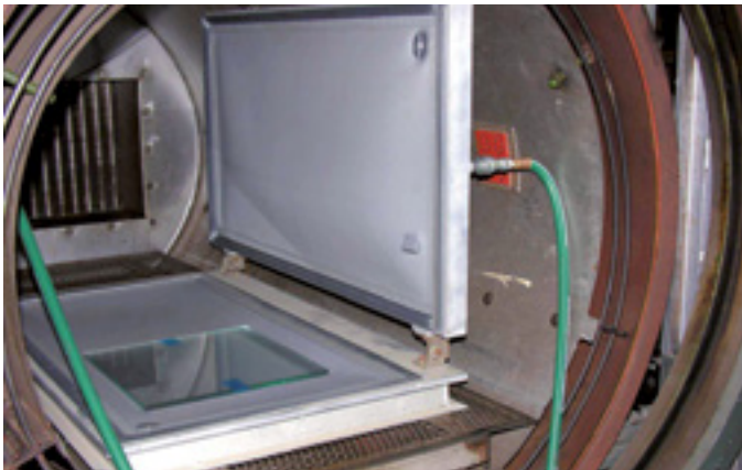
FIG 21 • Clamshell assembly (reusable)
